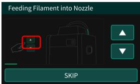
Wait for the extruder module to be heated to the working temperature after confirming that the filament is loaded, which will be driven by the feeding system to push the extruder module along the filament tube; or directly press and hold the "up" key to speed up the feeding.
