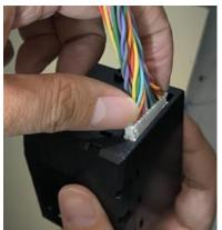
Mind the pinching position (as shown in the figure) when inserting the heating cable into the interface, and confirm the fool-proof position, then align the two ends and insert with even force.
