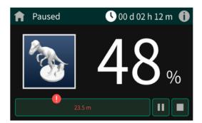
Click the "filament data button" on the screen to check filament status, or click this button (filament data button) to access the "replace filament" function when there is a reminder of insufficient filament.
