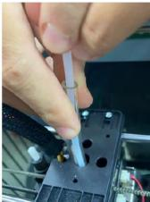
Guide tube clips (This file is stored on USB drive) and Top cover buckle Installation
