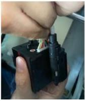
Mind the pinching position (as shown in the figure), and pull out the heating cable with even force.
