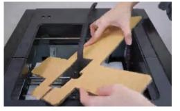
8. Remove the tape on the fixing cushions on the left and right sides, and remove all cushions inside the machine.
