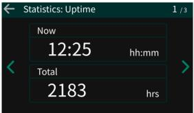
Uptime: Display the cumulative time of this use and the total cumulative time after the machine is started and used.
