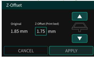
Wait for the extruder module to automatically move to the adjusted position, check the distance between the nozzle and the print bed after positioning, and then evaluate the height of Z axis to be adjusted. It is recommended to adjust the nozzle to the position touching the print bed. Click "Apply" to save the settings after the adjustment.
