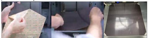
After that, load the Removable metal print bed (Accessory 11) on the magnetic-bonded print bed.
